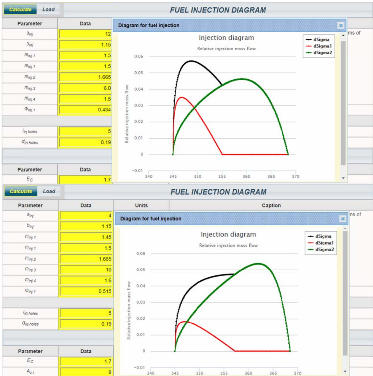
Fig. 2.4.4. Fuel injection diagrams for different sets of adjustable factors in the Razlejtzev approximating equations. Black line indicates the total fuel injection rate d\sigma/d\phi , red and green – first d\sigma/d\phi_1 and second d\sigma/d\phi_2 functions respectively.
